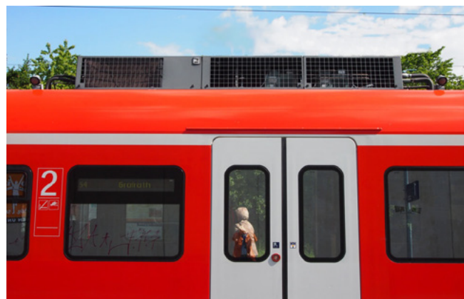
Figure 4: Air-conditioning system on a train roof.
