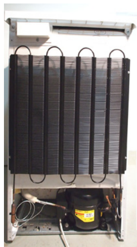
Figure 2: The back of a refrigerator. One can see the pipes for the coolant and the "cooling fins" as well as the compressor (at the bottom).
