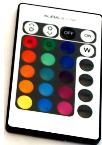
Fig. 7: Control panel for mixing the colored living room lighting.
